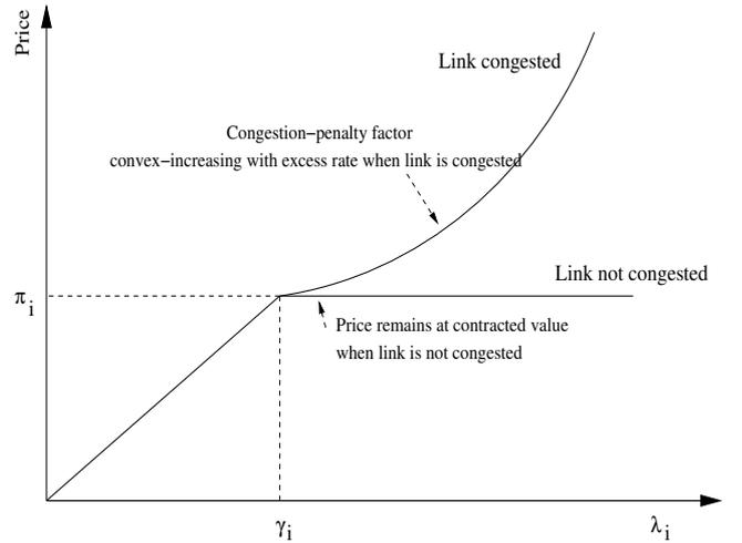
Fig. 3. Schematic showing how the price charged by the SP changes, depending on both the rate at which a user sends traffic and the state of congestion of the link.
