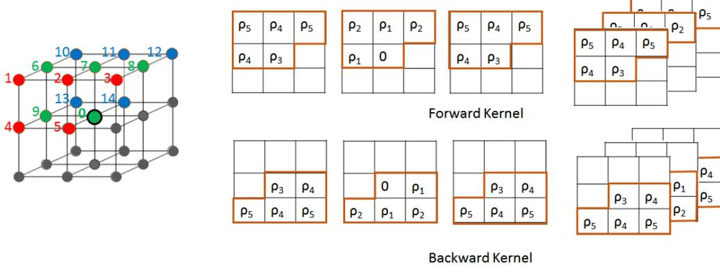
Figure 2. Kernel for 3D geodesic distance transform.
